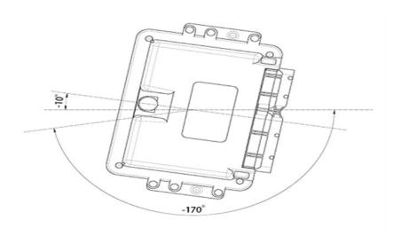
ECOTRON recommends using the six mounting holes on the VCU for installation. It is recommended to use metal materials such as aluminum alloy for the mounting bracket. The housing should have a reliable electrical connection with the vehicle body through the bracket.
