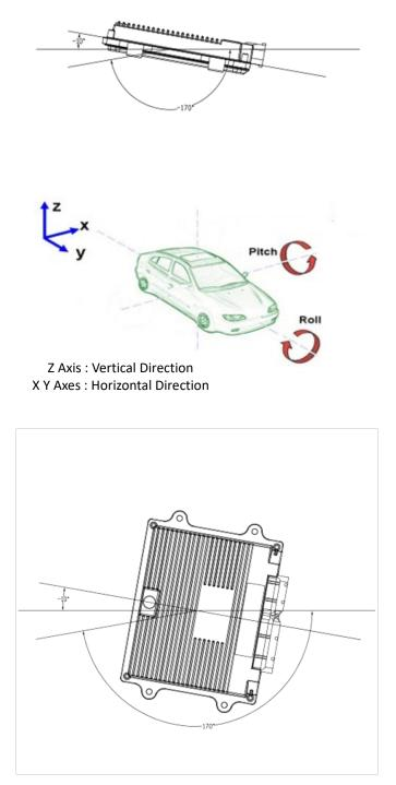
ECOTRON recommends using the four mounting holes on the FCU for installation. It is
