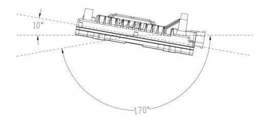
Ecotron recommends using the 4 mounting holes on the ADCU for installation. It is recommended to manufacture the mounting bracket out of metal materials such as aluminum alloy, and the housing should have a reliable electrical connection with the vehicle GND through the bracket. If other materials are used, the customer must ensure that it can meet the requirements of ADCU for vibration, heat dissipation, temperature, EMC, etc. If there is any deviation, it needs to be confirmed with Ecotron.
