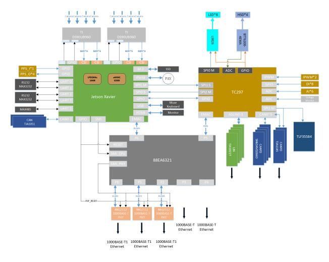
The internal circuit structure of EAXVA04 is shown below:
