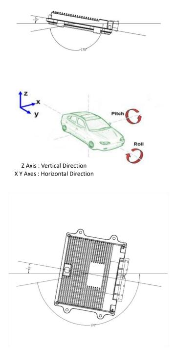
ECOTRON recommends using the four mounting holes on the VCU for installation. It is
