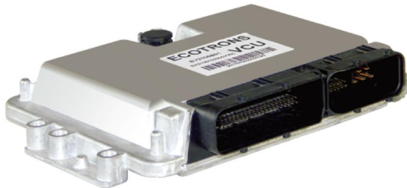
Figure 2 VCU Housing Appearance
