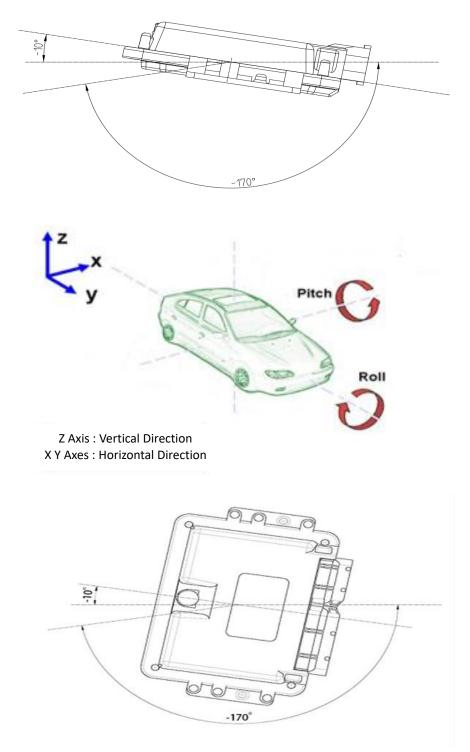
ECOTRON recommends using the six mounting holes on the VCU for installation. It is
