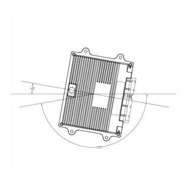
ECOTRON recommends using the four mounting holes on the FCU for installation. It is recommended to use metal materials such as aluminum alloy for the mounting bracket. The housing should have a reliable electrical connection with the vehicle body through the bracket.
