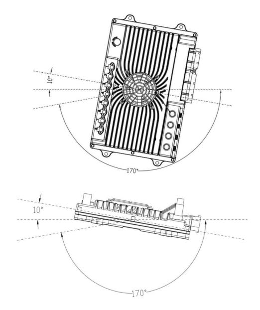
Ecotron recommends using the 4 mounting holes on the ADCU for installation. It is recommended to manufacture the mounting bracket out of metal materials such as aluminum alloy, and the housing should have a reliable electrical connection with the vehicle GND through the bracket. If other materials are used, the customer must ensure that it can meet the requirements of ADCU for vibration, heat dissipation, temperature, EMC, etc. If there is any deviation, it needs to be confirmed with Ecotron.
