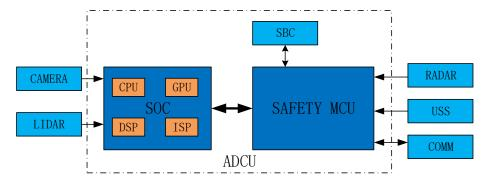
SoC (System on Chip) primarily handles tasks such as camera image data processing, laser radar point cloud data processing, and the generation of an output target recognition list through deep learning algorithms. It can also be used for sensor fusion, trajectory prediction, and other advanced functions.
