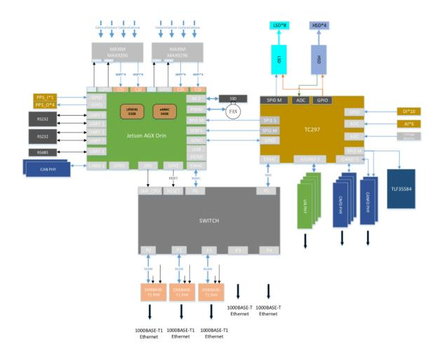
SOC is based on a GPU+CPU architecture, excelling in "large-scale and low precision" floating-point operations. It serves as the primary processing unit for perception tasks, including the processing of data from front-view, side-view, surround-view cameras, lidar, and inertial navigation systems.
