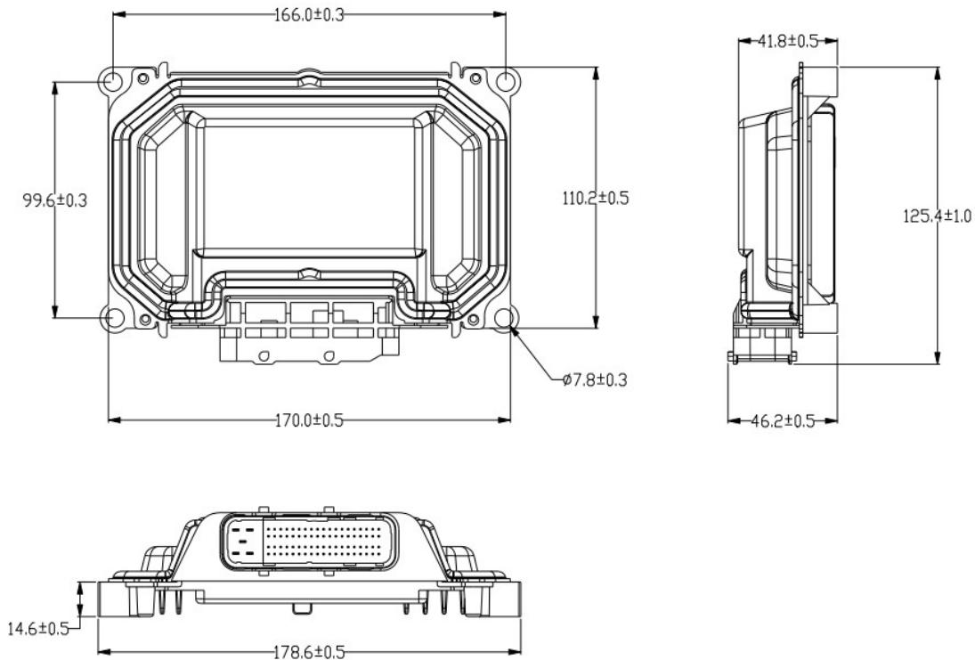
Figure 1 VCU Housing Size
