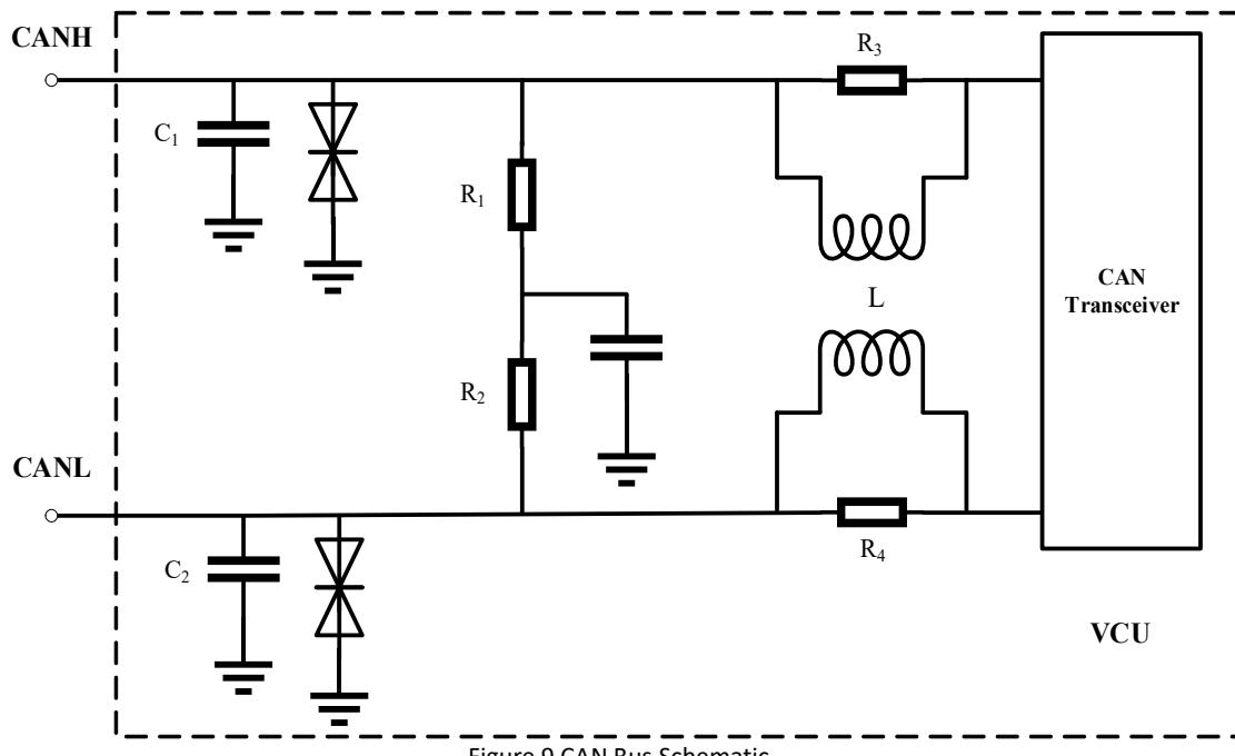
Figure 9 CAN Bus Schematic
