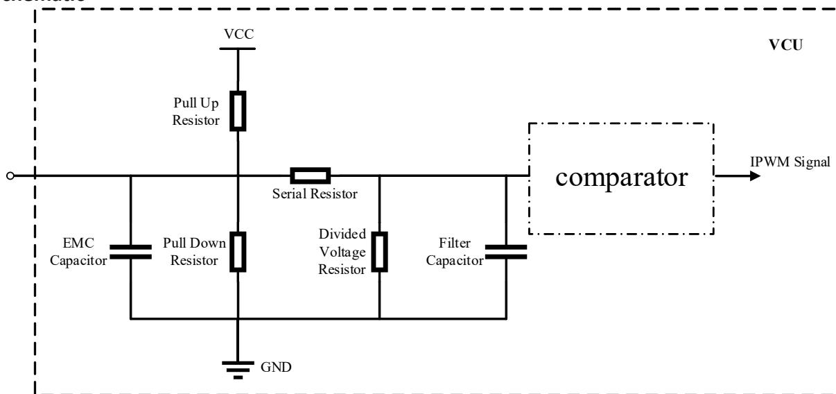
Figure 6 Schematic Diagram of Frequency Signal Input Channel
