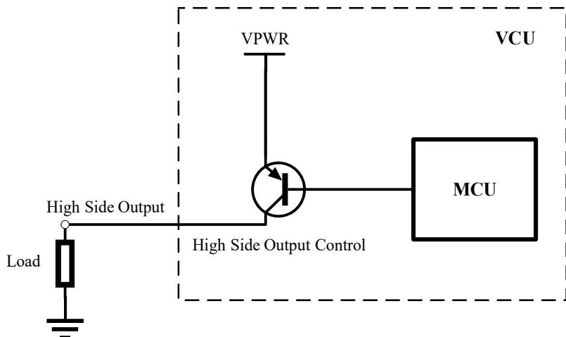
Figure 8 Schematic Diagram of High-Side Driver Channel
