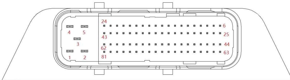
Figure 3 Connector's Pin Distribution Diagram
