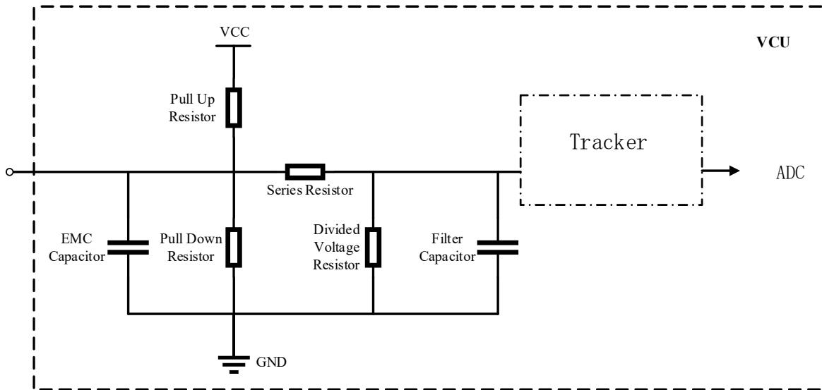
Figure 4 Schematic of Analog Signal Input Channel
