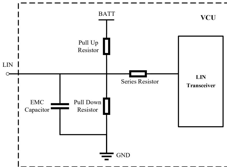
Figure 10 LIN Bus Schematic
