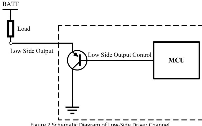
Figure 7 Schematic Diagram of Low-Side Driver Channel
