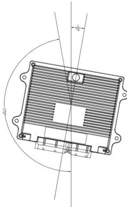
Figure 14 Vertical Installation Angle
