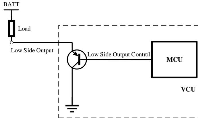
Figure 8 Schematic Diagram of Low-Side Driver Channel
