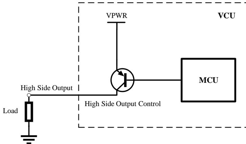
Figure 9 Schematic Diagram of High-Side Driver Channel
