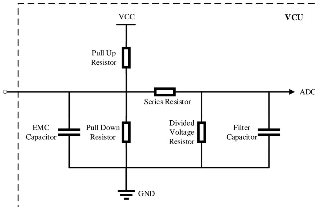
Figure 4 Schematic of Analog Signal Input Channel
