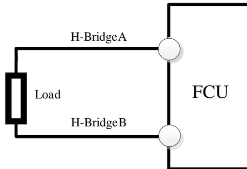
Figure 7 H-bridge Working Principle
