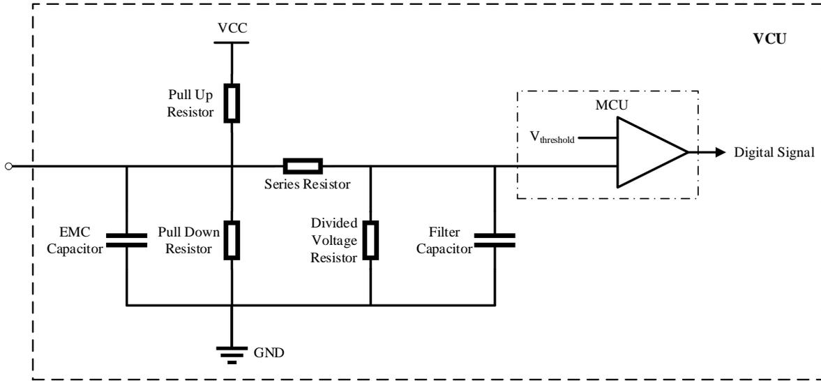
Figure 5 Schematic of Digital Signal Input Channel
